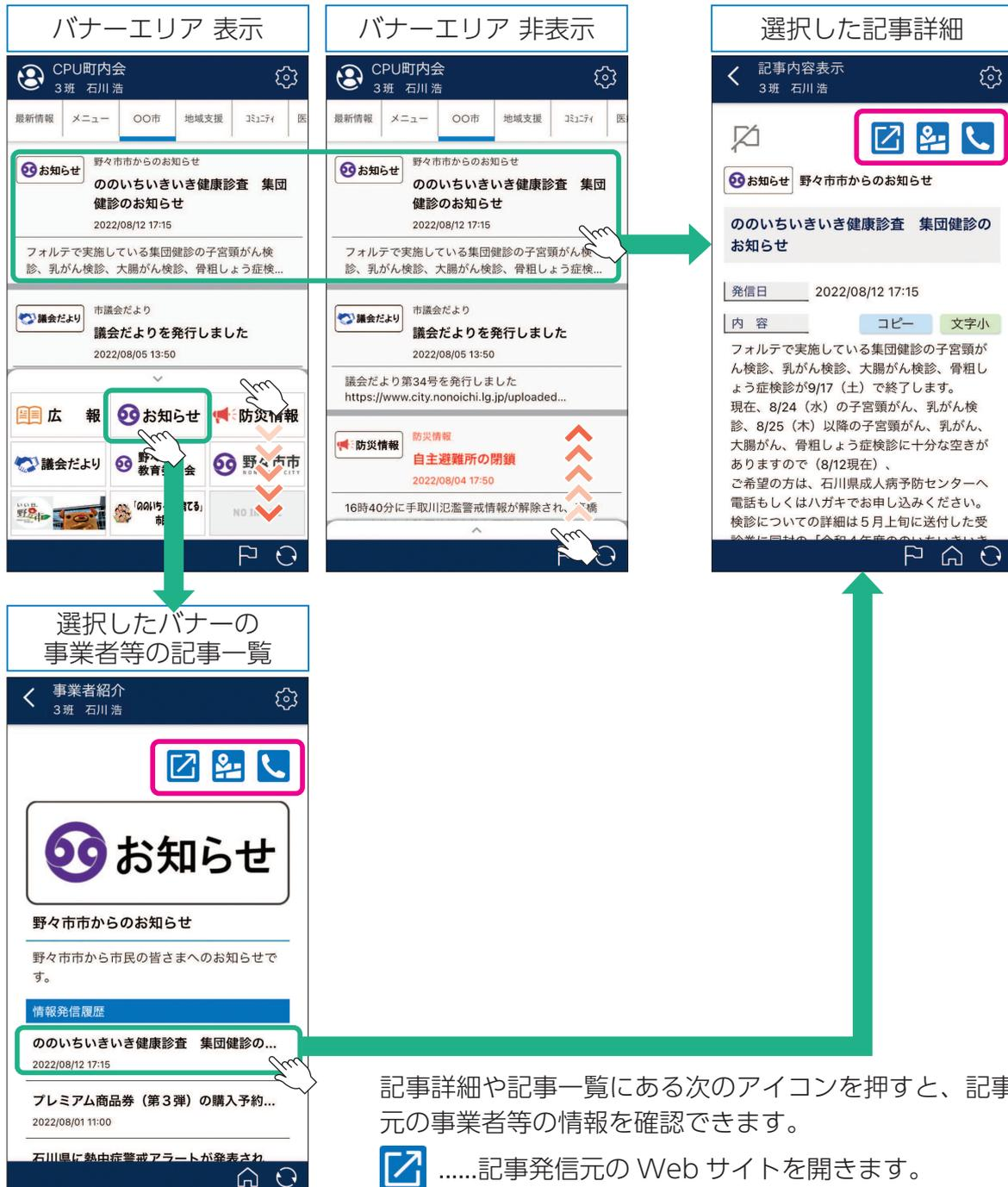
The diagram illustrates the user flow for interacting with a banner. It starts with a main screen where a banner is visible. Pressing the banner leads to a list of articles from the same sender. From this list, pressing an article leads to its detailed view. In the detailed view, there are three icons: a link icon, a location pin icon, and a phone icon. Pressing these icons provides additional information about the sender.
